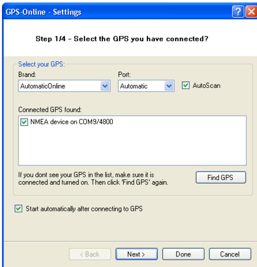
On the first page of the assistant select the GPS-unit. If the button **AutoScan** is activated, QV tries to find a connected unit automatically. Accordingly to the selection all units are searched and displayed
